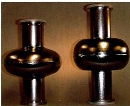
Fig. 1. Comparison of the TESLA cavity shape (left) and the new cavity shape.
