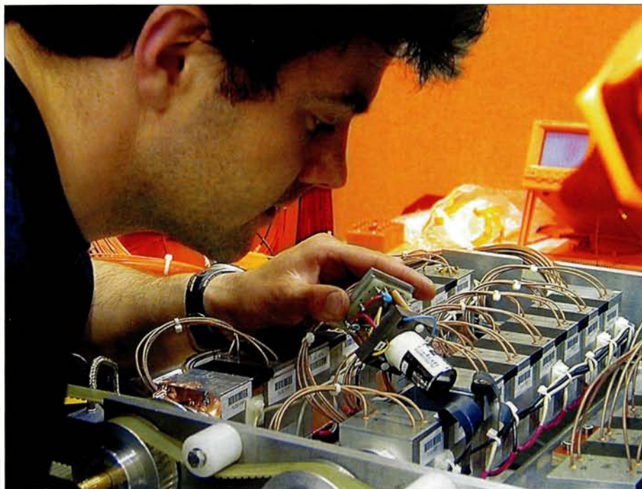
Joolz Williams working on the vacuum phototriode testing system at the Rutherford Appleton Laboratory. CMS will ultimately use 15 500 VPTs. (Courtesy CCLRC RAL.)
