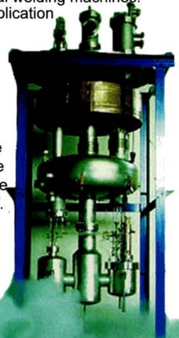
Superfluid helium cryostat working at 1.8 K
