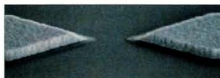
Top: schematic illustration of the structure of the NMR device, based on a 20 nm gallium arsenide quantum well. A pair of Schottky split gates defines the point contact channel, indicated by a white ellipse. Bottom: scanning electron microscope image of the split gates beneath the antenna gate. The gap between the gates is 600 nm.
